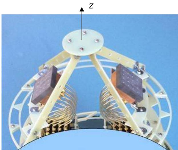
Fig. 1. A scaled generic model with two subarrays symmetrically positioned.
